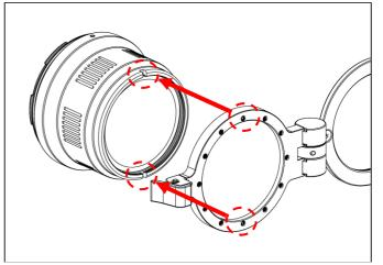
Align the two positioning screws on the back of the holder with the slots on the front of the port.
